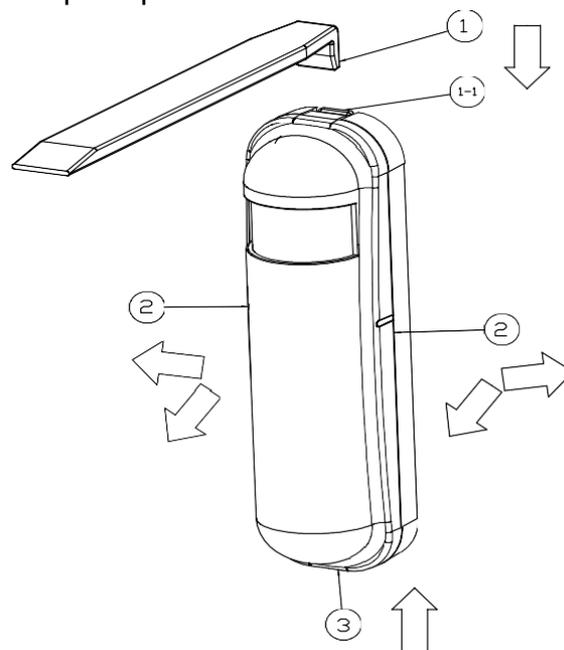
Replace the new battery and install the cover back.
